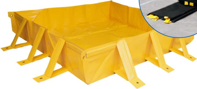
SpillSmart Collapsible Bunds provide cost-effective temporary storage for liquids and chemicals whilst containing potential spills and leaks. These Bunds are easy to store and quick to deploy. The external folding legs lock into place keeping the 300mm side walls rigid. Within seconds, the legs can be unlocked and folded down allowing access for pallet jacks, forklifts and vehicles. Eyelets are also provided on the base of the legs if pegging to soft ground is required.
